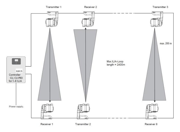
The illustrated components are examples and can be combined within the scope of the technical possibilities. The technical documentation, installation instructions and regional standards must be observed.
